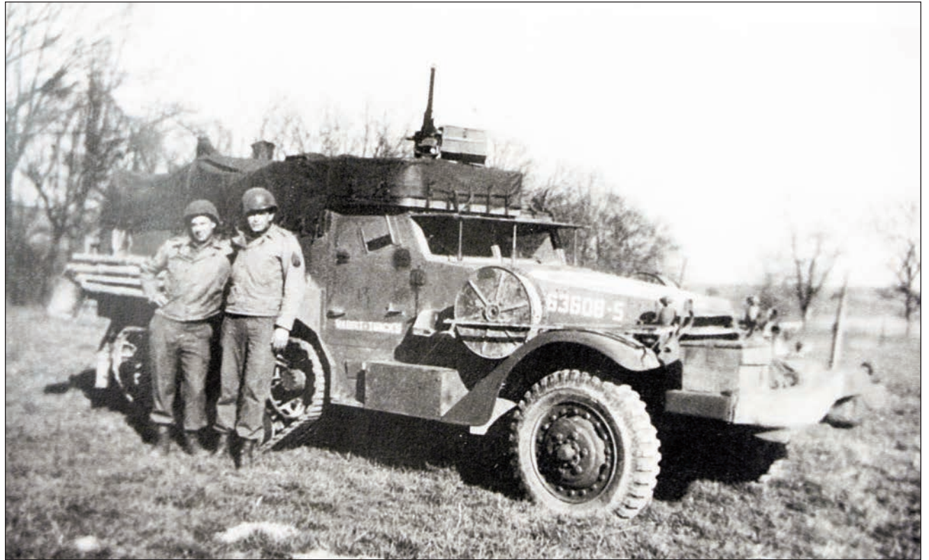
The 777th went to battle in halftracks, vehicles with wheels in front and treads in the rear. This halftrack was fitted out for headquarters duty and only had one mounted 50 caliber machine gun. Other halftracks either had four 50 calibers mounted in back, or two 50 calibers and an anti-aircraft cannon. The unit shot down 111 German planes in the war.
