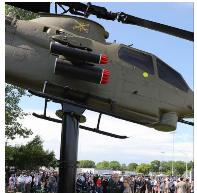
The Bell AH-1 Cobra has a two-blade rotor with a single engine and BGM-71 TOW anti-armor missiles. The Army used the attack copters in Vietnam from 1967 to 1973.
