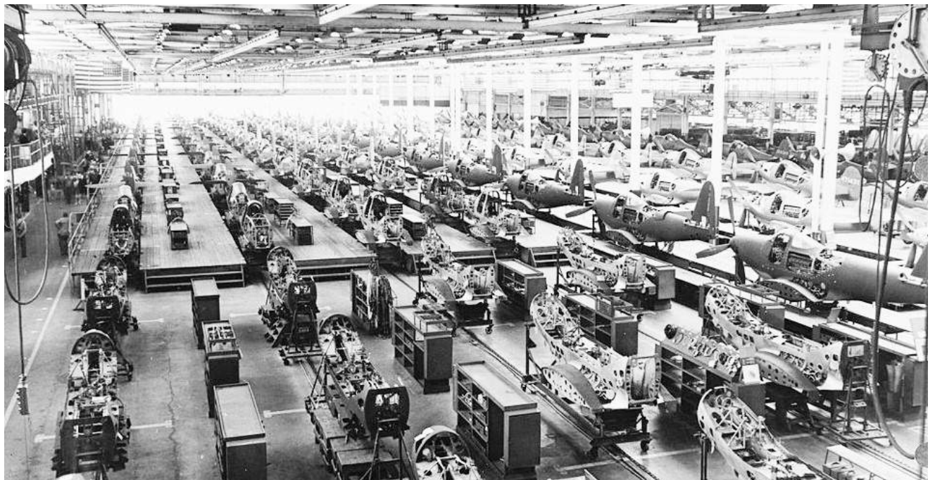
An assembly plant for fighter aircraft stretches into the distance in New York during World War II.
