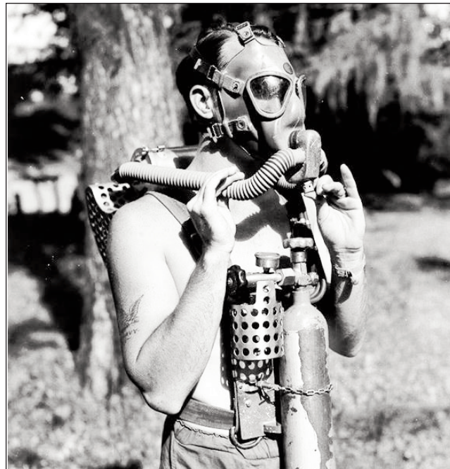
A diver tries out an early version of the LARU which recycled the air and produced no bubbles.
