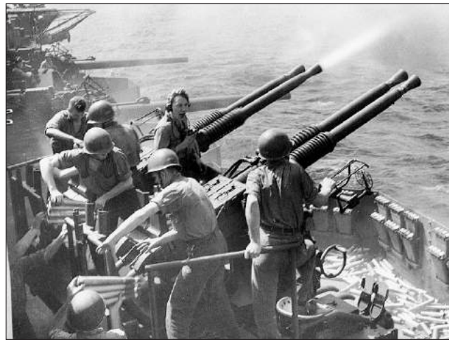
A Navy crew on the USS Hornet mans 40 mm guns similar to the ones Falk operated on the USS Darke. There were trainers, pointers and loaders. The man in the headset is probably the gunner's mate.
