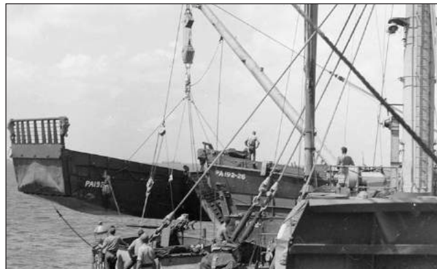
A crane on the transport ships could put four landing craft in the water in 14 minutes.
